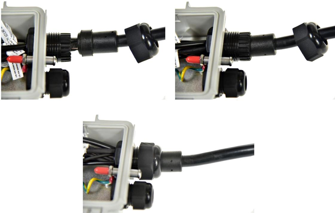
A network cable *without a protective cover* will fit easily through the second cable gland. If your cable has a protective cover or a latch guard you may need to remove it.
