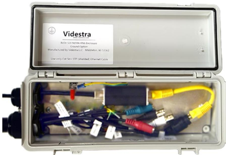
Insertion of the Bolin umbilical should be done carefully. Note that most cables with bare ends are capped and should remain so.
