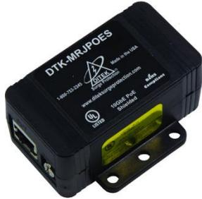
connection from the surge suppressor to the camera is STP (Shielded Twisted Pair) and not simply UTP (Unshielded Twisted Pair). A surge suppressor will not help if that link is not providing a path to ground. You may use UTP cable *after* the surge suppressor as the suppressor itself will provide its own path to ground.
