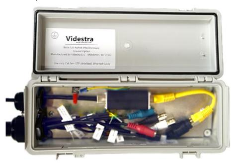
Insertion of the Bolin umbilical should be done carefully. Note that most cables with bare ends are capped and should remain so.
