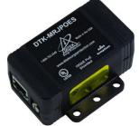
connection from the surge suppressor to the camera is STP (Shielded Twisted Pair) and not simply UTP (Unshielded Twisted Pair). A surge suppressor will not help if that link is not providing a path to ground. You may use UTP cable *after* the surge suppressor as the suppressor itself will provide its own path to ground.
